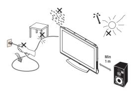
Ensure that the TV is placed in a position to allow free flow of air. Do not cover the ventilation openings on the back cover. To prevent any unsafe situations, no naked flame sources, such as lighted candles, should be placed on or in the vicinity. Avoid heat, direct sunlight and exposure to rain or water. The equipment shall not be exposed to dripping or splashing.
